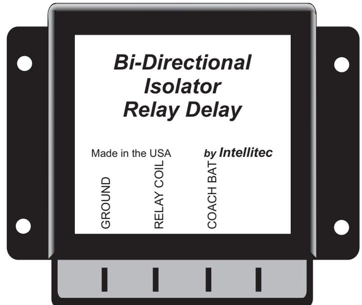
After the solenoid has been closed, the system continues to sense the voltage. If the ignition switch is off and the battery voltage drops below 12.8 volts for approximately 5 seconds, which might occur when the converter is heavily loaded, the solenoid is opened to prevent the chassis battery from being discharged by the coach loads. When the voltage goes above 13.4 volts again for approximately 5 seconds, the solenoid closes again.
